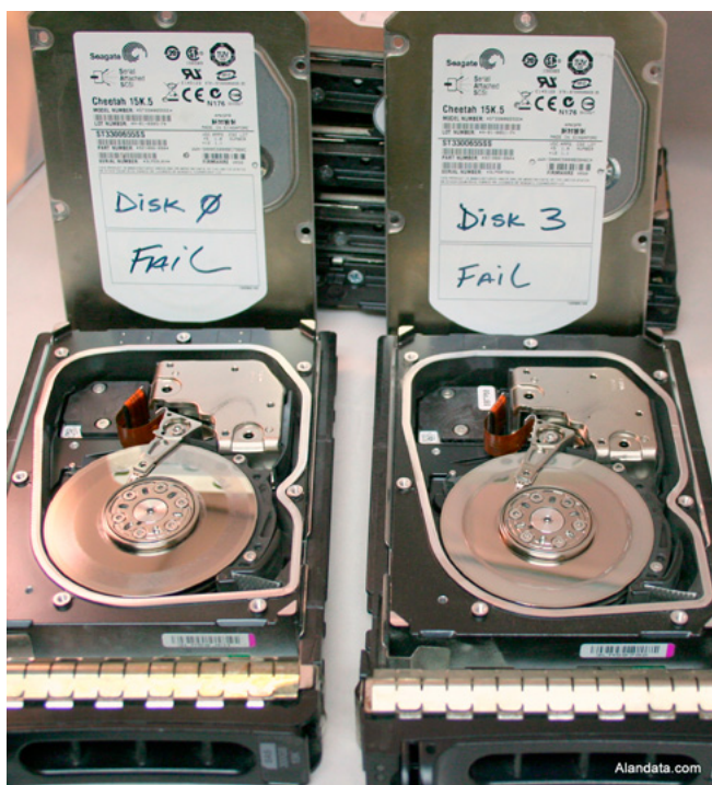
Figure 1. Two failed hard drives after RAID
